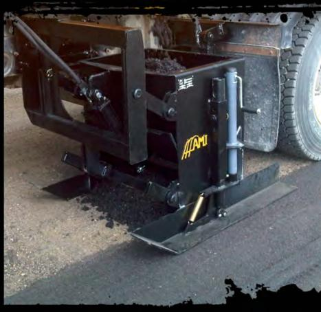
"Using two Pavement Edgers, we shouldered over 10 kilometers of new pavement directly behind the asphalt crew in less than 2 full working days."
