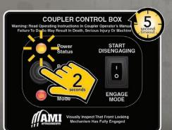
**1.** Start the process by switching the engage mode on. The power status signal indicates that power is on accompanied by a continuous audio alarm.
