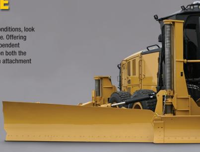
With up to a 12 ft. wide mouldboard, extendible push pole with 25" extension, and a control valve with in-cab joystick controls, this blade assembly is designed for efficient snow removal and user-friendly setup. The Wing Blade provides an impressive 48" of level bench height and comes equipped with a reversible bolt-on edge.
