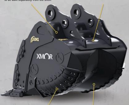
Being mechanically attached, the bolt-on heel shrouds reduce service maintenance time as well as reduce steel overlap for a lighter bucket. The Inverted Keel is a proven and unique XMOR® feature serving the dual purpose of distributing the material smoothly inside the bucket and keeping the external plate away from the material, thus reducing wear.
