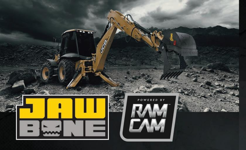
When multi-tasking is a must, the AMI Attachments Jawbone 4-in-1 Excavator Bucket Powered by RAMCAM responds with a multipurpose design that digs, grades, grips and clamshells. The RAMCAM technology works using hydraulic cylinders which are fully enclosed and fully protected from the elements.
