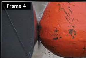
Frame 4 shows maximum steel deflection from 22,000 ft-lbs of energy impacting the PRO+ bucket, captured at 120 frames per second.
